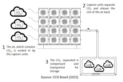
Figure - 4 Illustration of the path taken by CO<sub>2</sub> molecules from capture to storage in a DAC unit.
