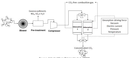
Figure - 5 Conventional flowchart of CO<sub>2</sub> separation by adsorption.
