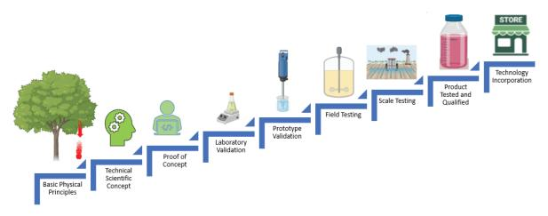
Figure - 6 The nine levels of technological maturity, Technology Readiness Level (TRL).
