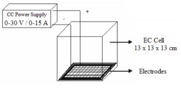
Figure 1 - Bench-scale EC reactor.
